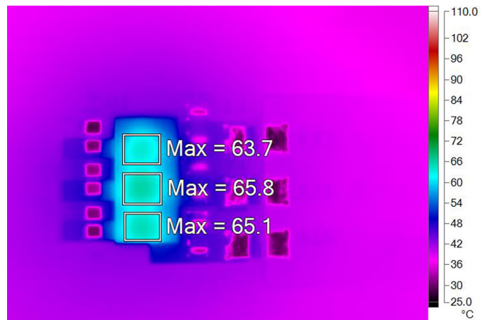
Figure 5. Thermal Image, Full Load with Three Channels in Parallel (1.3 V_{IN} , 1 V_{OUT} , 9A) without Fan, T_A = 25^\circ\text{C}
