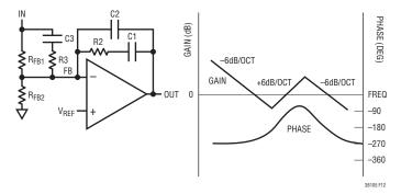
Figure 12. Type 3 Schematic and Transfer Function
