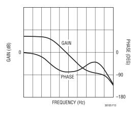
Figure 13. Transfer Function of Buck Modulator
