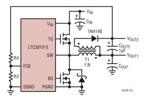
Figure 14. Secondary Output Loop
