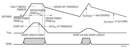
Figure 10. Fault Timeout Operation
