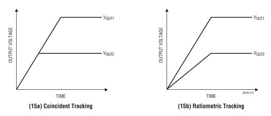
Figure 15. Two Different Modes of Output Voltage Tracking
