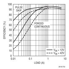
Figure 2. Efficiency in Pulse Skip/ Forced Continuous Modes
