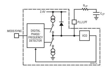
Figure 18. Phase-Locked Loop Block Diagram
