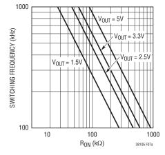
Figure 7a. Switching Frequency vs  $R_{ON}$  ( $V_{ON} = OV$ )
