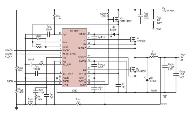
Figure 19. 12V to 60V Input Voltage to 5V/6A Synchronized at 250kHz
