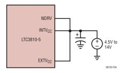
Figure 4. Operating Modes for IC/Driver Supply
