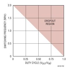
Figure 9. Maximum Switching Frequency vs Duty Cycle
