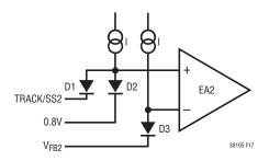
Figure 17. Equivalent Input Circuit of Error Amplifier
