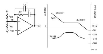
Figure 11. Type 2 Schematic and Transfer Function
