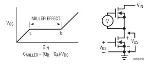
Figure 6. Gate Charge Characteristic
