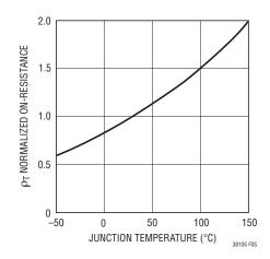
Figure 5. R<sub>DS(ON)</sub> vs Temperature
