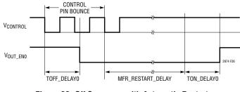
Figure 26. Off Sequence with Automatic Restart
