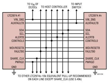
Figure 29. Typical Connections between Multiple LTC2974s
