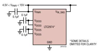
Figure 23. Powering LTC2974 Directly from an Intermediate Bus
