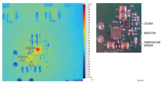
Figure 40. Thermal Image of a DC/DC Converter Showing the Difference Between the Actual Inductor Temperature and the Temperature Sensing Point
