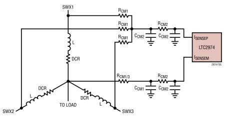
Figure 35. Multiphase DCR Current Sensing Circuits
