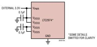
Figure 24. Powering LTC2974 from External 3.3V Supply
