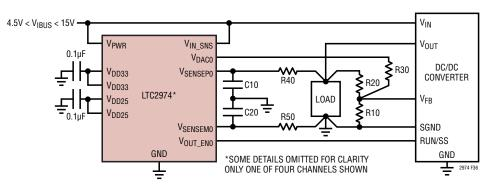
Figure 36. Anti-Aliasing Filter on  $V_{\mbox{SENSE}}$  Lines
