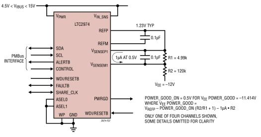
Figure 37. Sensing Negative Voltages
