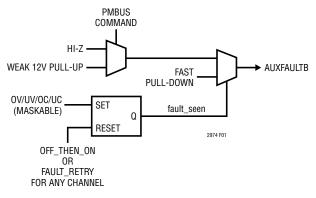
Figure 1: AUXFAULTB MUX
