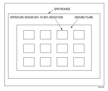
Figure 42. Suggested Screen Pattern for Die Attach Pad
