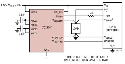
Figure 32. Application Circuit for DC/DC Converters with Trim Pin
