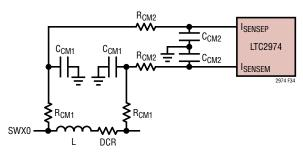
Figure 34. DCR Current Sensing Circuits
