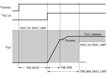
Figure 25. Typical ON Sequence Using Control Pin
