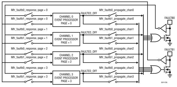
Figure 28. Channel Fault Management Block Diagram
