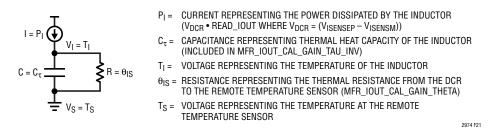
Figure 21. Electronic Analogy for Inductor Temperature Model
