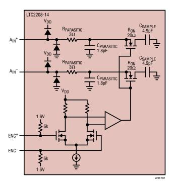
Figure 2. Equivalent Input Circuit
