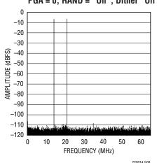
32k Point 2-Tone FFT, f<sub>IN</sub> = 20.14MHz and 14.25MHz, -25dBFS, PGA = 0, RAND = "On", Dither "Off"
