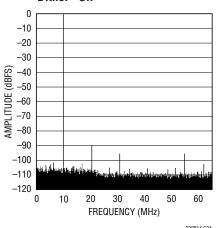
SFDR vs Input Level,  $f_{IN} = 140.1MHz$ , PGA = 1, RAND = "On", Dither "Off"
