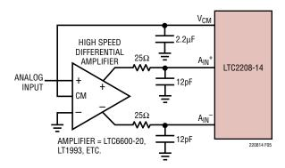
Figure 5. DC Coupled Input with Differential Amplifier
