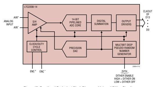
Figure 15. Functional Equivalent Block Diagram of Internal Dither Circuit
