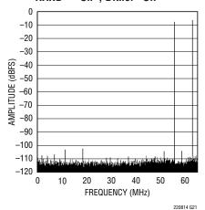
32k Point 2-Tone FFT,  $f_{IN} = 67.2MHz$ and 74.4MHz, -15dBFS, PGA = 0, RAND = "On", Dither "Off"
