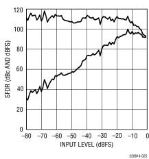
SFDR vs Input Level,  $f_{IN} = 140.1MHz$ , PGA = 1, RAND = "On", Dither "On"
