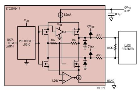
Figure 12. Equivalent Output Buffer in LVDS Mode
