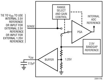
Figure 6. Reference Circuit
