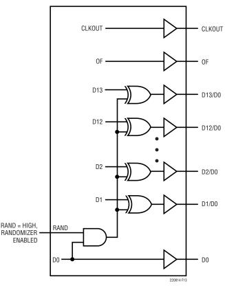
Figure 13. Functional Equivalent of Digital Output Randomizer
