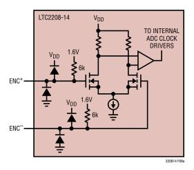
Figure 8a. Equivalent Encode Input Circuit
