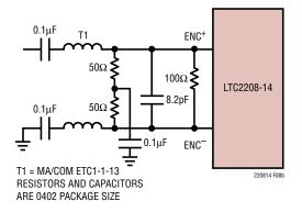
Figure 8b. Transformer Driven Encode
