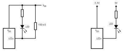
Figure 11. Methods to Reduce  $I_Q$  When LEDs are in OFF State
