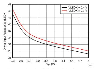
Figure 12. Typical LED Switch Resistance
