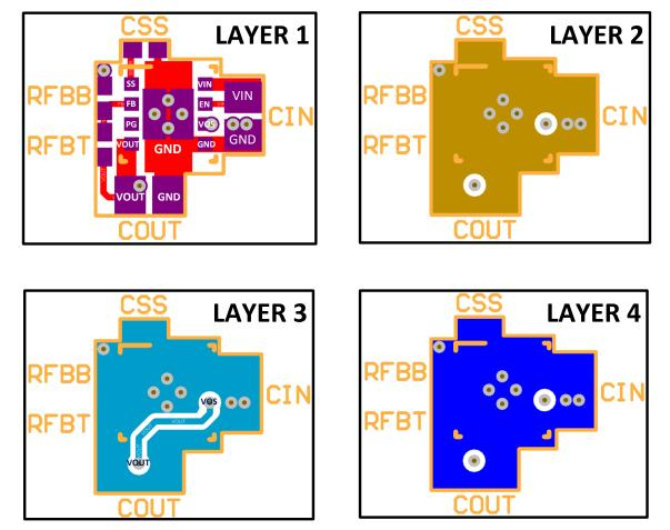
Figure 82. 35 mm<sup>2</sup> Solution Size (Single Sided)
