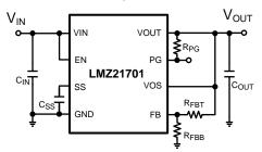
Figure 14. Typical Applications Circuit
