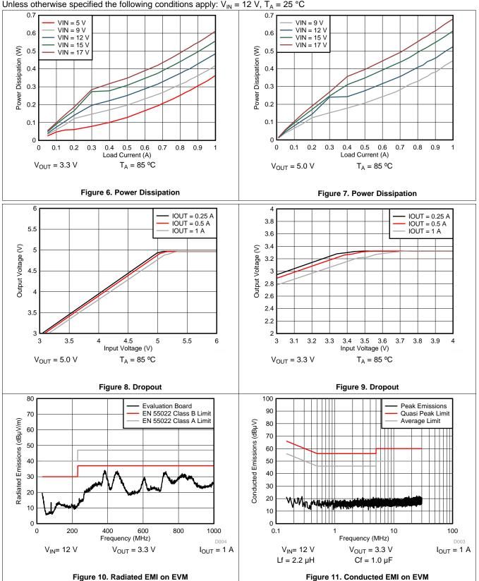
Unless otherwise specified the following conditions apply:  $V_{IN}$  = 12 V,  $T_A$  = 25 °C
