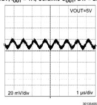
Output Ripple  $V_{IN}$  = 24V,  $I_{OUT}$  = 1A, Polymer Electrolytic  $C_{OUT}$ , BW = 200 MHz
