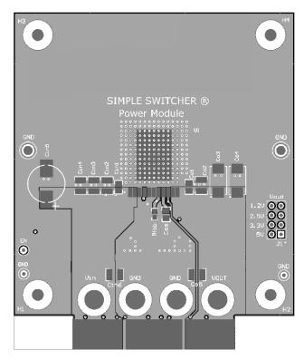
Figure 55. Top View of Evaluation PCB
