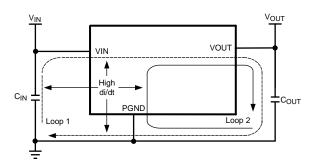
Figure 53. Critical Current Loops to Minimize
