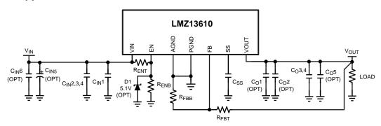
Figure 47. Typical Application Schematic
