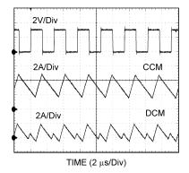
$V_{IN}$  = 12 V,  $V_{O}$  = 3.3 V,  $I_{O}$  = 3 A / 0.3 A
