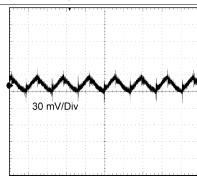
$\label{eq:time} \text{TIME (2 }\mu\text{s/Div)}$  12  $V_{\text{IN}}$ , 5  $V_{\text{OUT}}$  at Full Load, BW = 250 MHz
