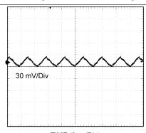
$\label{eq:time} \text{TIME (2 }\mu\text{s/Div)}$  12  $V_{\text{IN}},$  5  $V_{\text{OUT}}$  at Full Load, BW = 20 MHz
