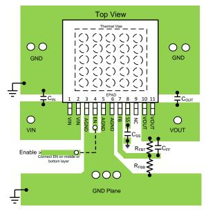
Figure 54. PCB Layout Guide
