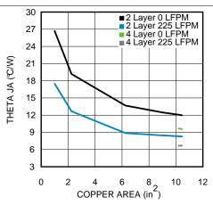
Figure 32.  $\theta_{\text{JA}}$  vs Copper Heat Sinking Area
