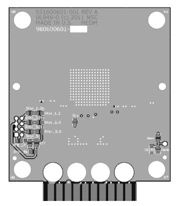
Figure 56. Bottom View of Evaluation PCB
