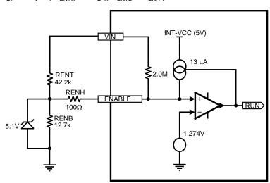
Figure 48. Enable Input Detail
