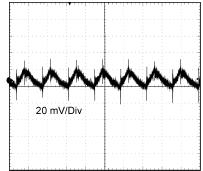
$\label{eq:time} \begin{aligned} &\text{TIME (2 }\mu\text{s/Div)} \\ \text{12 }V_{\text{IN}}, \, 3.3 \,\, V_{\text{OUT}} \,\, \text{at Full Load, BW} = 250 \,\, \text{MHz} \end{aligned}$
