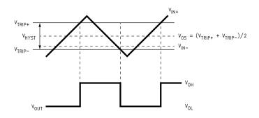
Copyright © 2016, Texas Instruments Incorporated Figure 19. Input and Output Waveforms, Non-Inverting Input Varied
