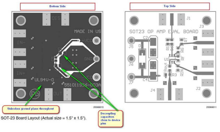
Figure 20. SOT-23 Board Layout Example
