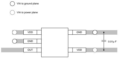
Figure 19. SC70 Package Recommended Layout
