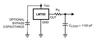
Figure 11. LMT85 with Series Resistor for Capacitive Loading Greater Than 1100 pF
