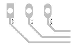
Figure 21. TO-92 LPM Package Recommended Layout
