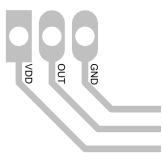
Figure 20. TO-92 LP Package Recommended Layout
