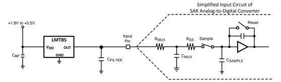
Figure 12. Suggested Connection to a Sampling Analog-to-digital Converter Input Stage
