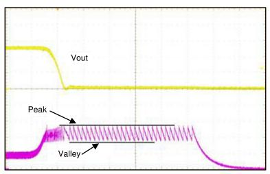
Figure 8-3. Current Limit Operation
