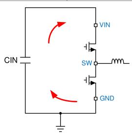
Figure 11-1. Current Loops with Fast Transients
