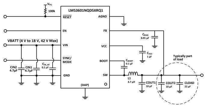
Figure 9-12. Typical LM53601NQDSXRQ1 Application Schematic
