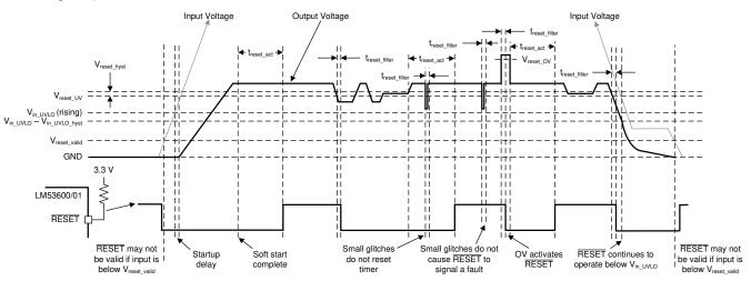
Figure 8-5. Reset Output Function Operation
