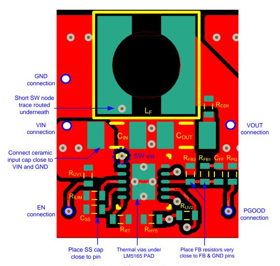
Figure 73. PCB Layout Example
