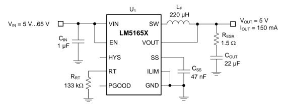
Figure 37. Schematic for Design 1 with V<sub>IN(nom)</sub> = 12 V, V<sub>OUT</sub> = 5 V, I<sub>OUT(max)</sub> = 150 mA, F<sub>SW(nom)</sub> = 230 kHz
