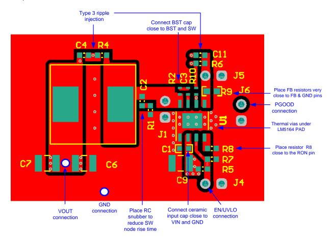
Figure 19. LM5164 Single-Sided PCB Layout Example
