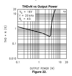
Typicals are measured at 25°C and represent the parametric norm.
