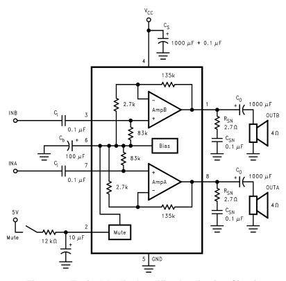
Figure 1. Typical Audio Amplifier Application Circuit
