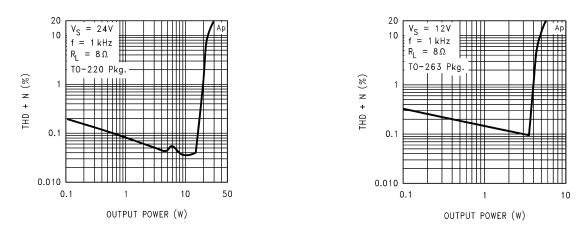
Figure 44. THD+N vs P<sub>OUT</sub> for Bridge-Mode Application
