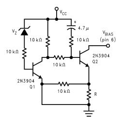
Figure 45. External Undervoltage Pull-Down
