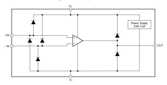
Figure 7-1. Equivalent Internal ESD Circuitry
