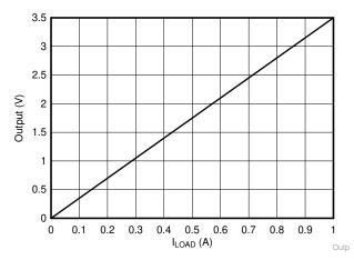
Figure 8-2. Low-Side, Current-Sense Transfer Function
