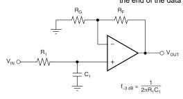
$$\frac{V_{OUT}}{V_{IN}} = \left(1 + \frac{R_F}{R_G}\right) \left(\frac{1}{1 + sR_1C_1}\right)$$
