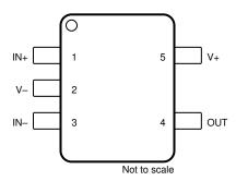
Figure 5-1. LM321LV DBV and DCK Package 5-Pin SOT-23 and SC70 (Top View)
