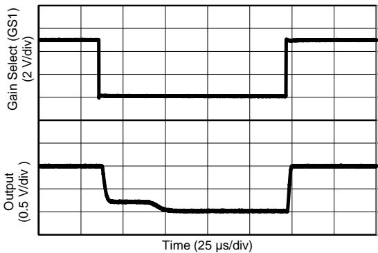
Figure 31. Gain Change Output Response From Saturation (Gain = 100 V/V to 25 V/V)
