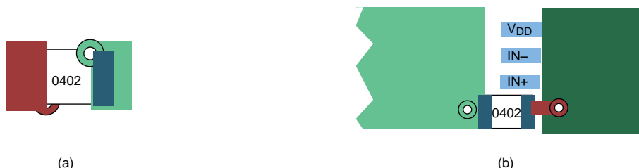
Figure 15. Typical Decoupling Capacitor Layouts
