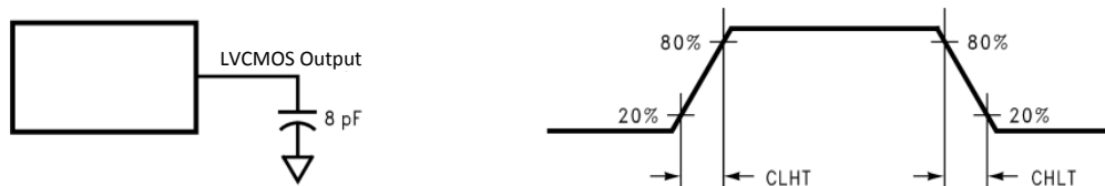
Figure 2. LVC MOS Output Load and Transition Times
