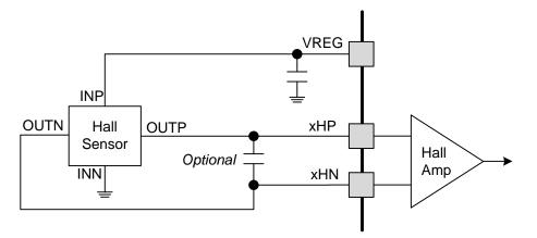
Figure 26. Hall Sensor Connections
