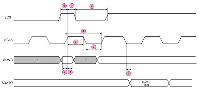
Figure 1. SPI Timing Requirements
