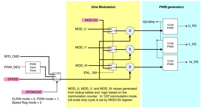
Figure 20. Modulation and PWM Generation
