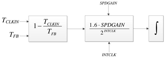
Figure 19. Integrator and Filters
