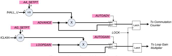
Figure 21. Auto Gain and Advance Functions
