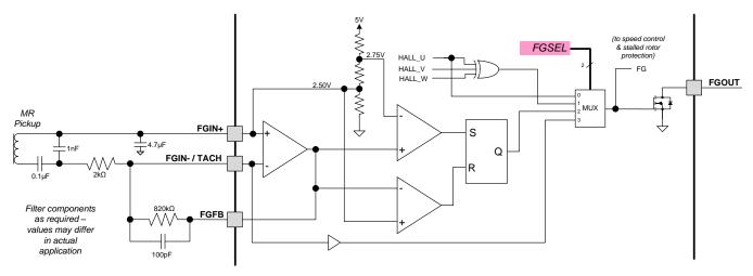
Figure 5. FG Circuit Diagram
