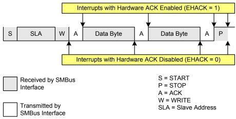
Figure 28.7. Typical Slave Write Sequence
