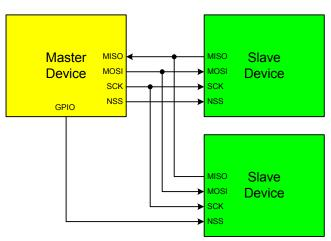
Figure 29.4. 4-Wire Single Master Mode and 4-Wire Slave Mode Connection Diagram
