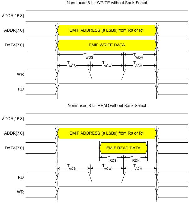
Figure 16.5. Non-multiplexed 8-bit MOVX without Bank Select Timing
