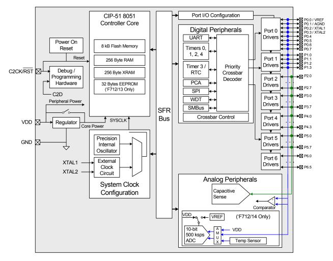
Figure 1.6. C8051F712/13/14/15 Block Diagram
