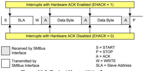
Figure 28.5. Typical Master Write Sequence
