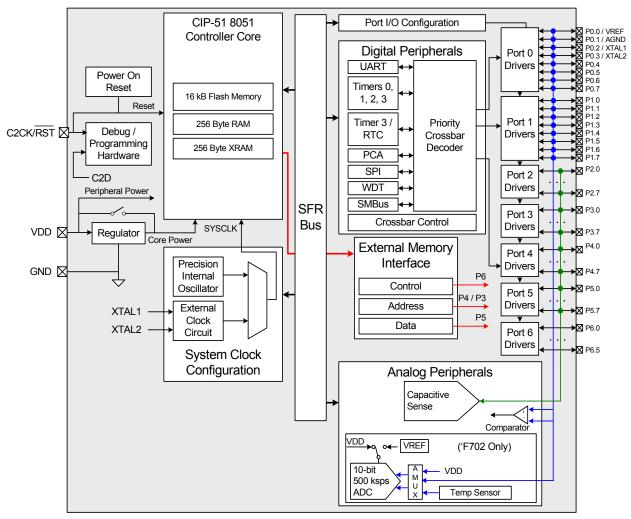
Figure 1.2. C8051F702/3 Block Diagram
