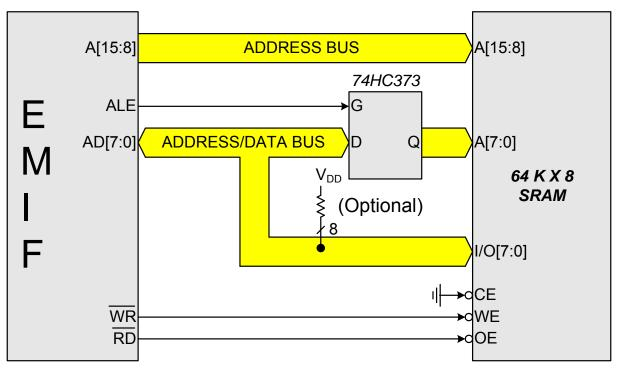
Figure 16.1. Multiplexed Configuration Example
