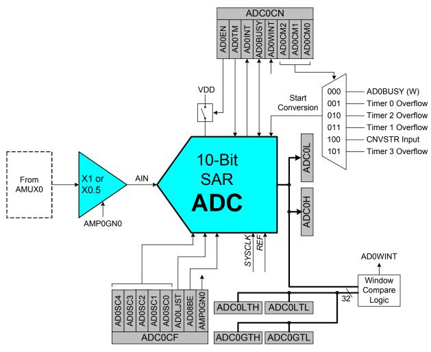
Figure 8.1. ADC0 Functional Block Diagram
