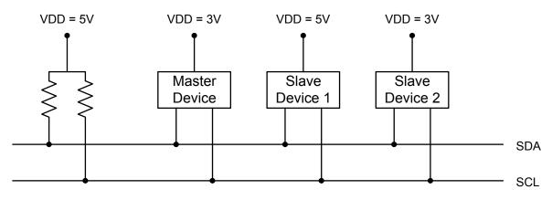
Figure 28.2. Typical SMBus Configuration
