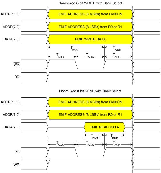
Figure 16.6. Non-multiplexed 8-bit MOVX with Bank Select Timing
