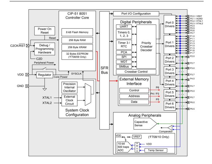
Figure 1.5. C8051F708/09/10/11 Block Diagram
