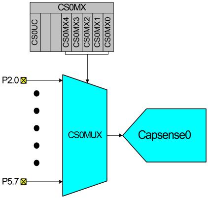
Figure 13.3. CS0 Multiplexer Block Diagram
