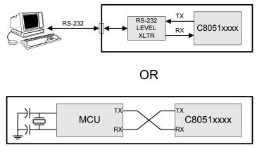
Figure 30.3. UART Interconnect Diagram
