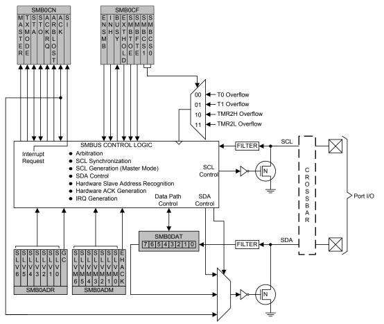
Figure 28.1. SMBus Block Diagram
