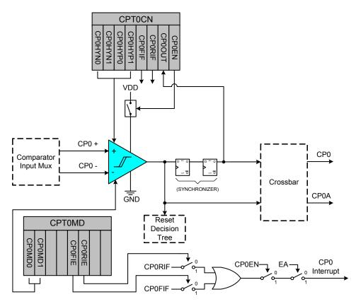
Figure 12.1. Comparator0 Functional Block Diagram
