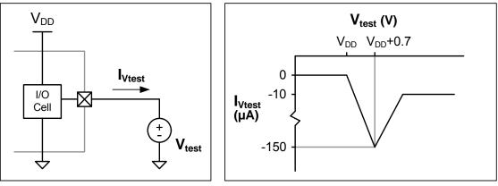
Port I/O Overdrive Test Circuit
