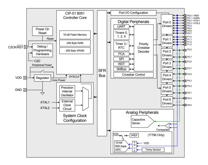
Figure 1.4. C8051F706/07 Block Diagram
