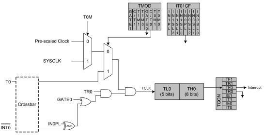
Figure 31.1. T0 Mode 0 Block Diagram
