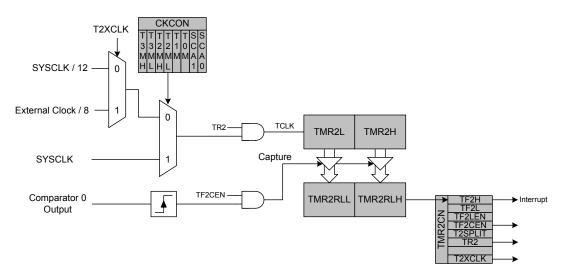
Figure 31.6. Timer 2 Capture Mode Block Diagram
