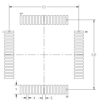
Figure 4.2. TQFP-64 PCB Land Pattern
