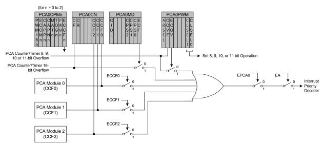
Figure 32.3. PCA Interrupt Block Diagram
