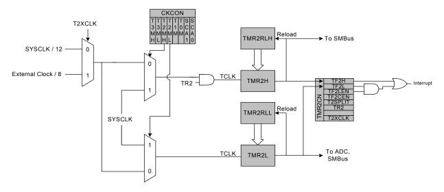
Figure 31.5. Timer 2 8-Bit Mode Block Diagram
