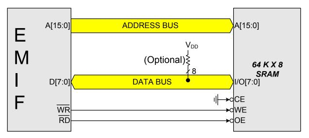
Figure 16.2. Non-multiplexed Configuration Example
