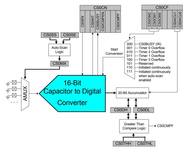
Figure 13.1. CS0 Block Diagram
