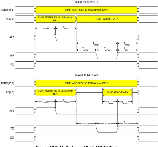
Figure 16.7. Multiplexed 16-bit MOVX Timing
