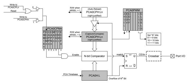
Figure 32.9. PCA 9, 10 and 11-Bit PWM Mode Diagram
