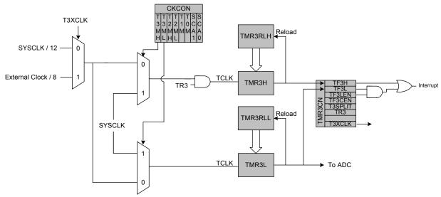
Figure 31.8. Timer 3 8-Bit Mode Block Diagram
