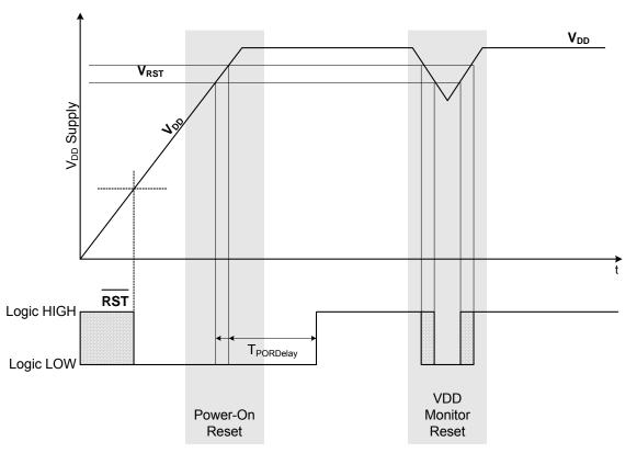
Figure 23.2. Power-On and V<sub>DD</sub> Monitor Reset Timing
