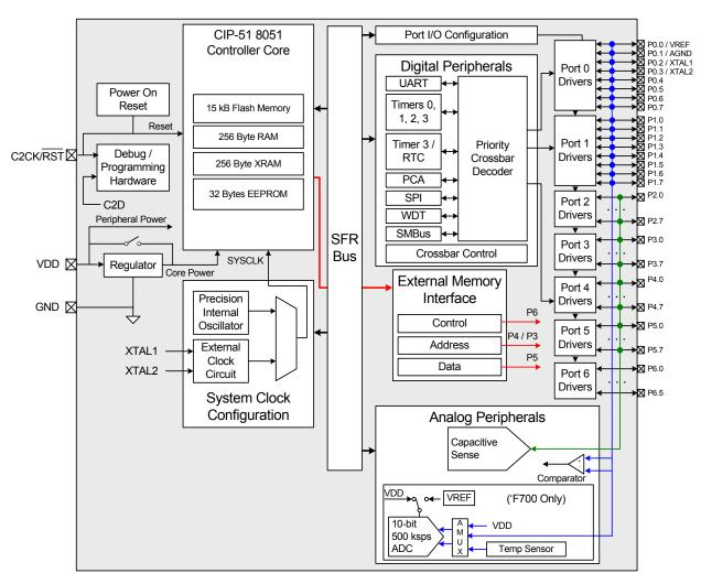
Figure 1.1. C8051F700/1 Block Diagram
