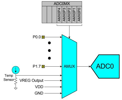
Figure 8.6. ADC0 Multiplexer Block Diagram
