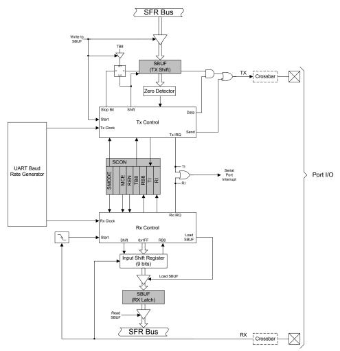
Figure 30.1. UART0 Block Diagram
