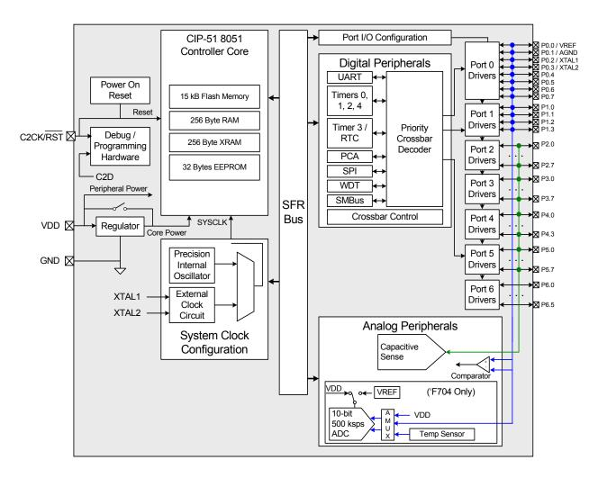
Figure 1.3. C8051F704/5 Block Diagram
