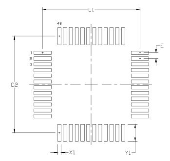
Figure 5.2. TQFP-48 PCB Land Pattern
