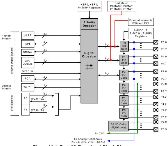
Figure 26.1. Port I/O Functional Block Diagram
