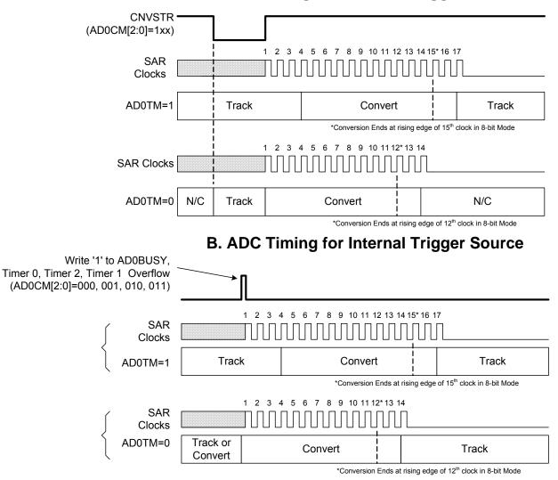
A. ADC Timing for External Trigger Source
