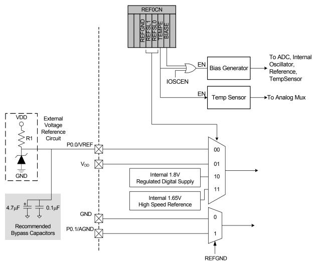
Figure 10.1. Voltage Reference Functional Block Diagram
