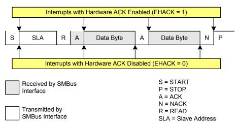
Figure 28.6. Typical Master Read Sequence
