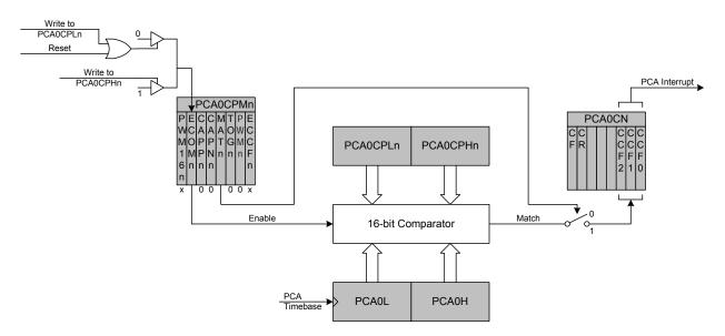
Figure 32.5. PCA Software Timer Mode Diagram
