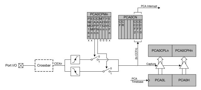
Figure 32.4. PCA Capture Mode Diagram
