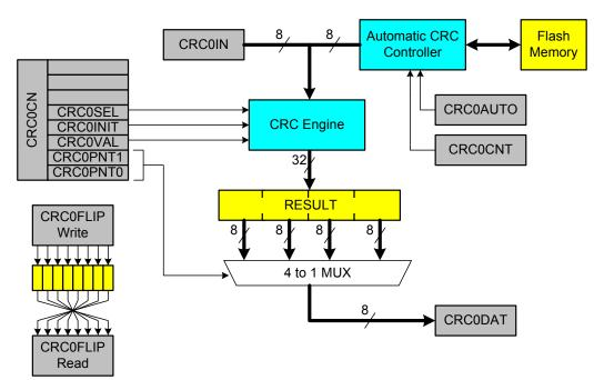
Figure 27.1. CRC0 Block Diagram
