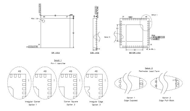
Figure 6.1. QFN-48 Package Drawing
