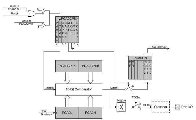
Figure 32.6. PCA High-Speed Output Mode Diagram
