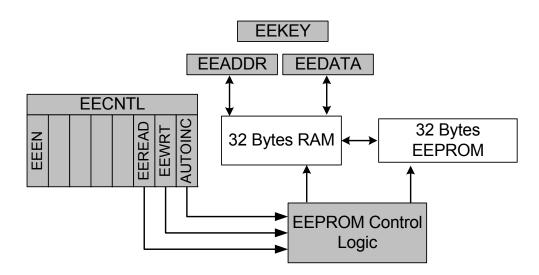
Figure 21.1. EEPROM Block Diagram
