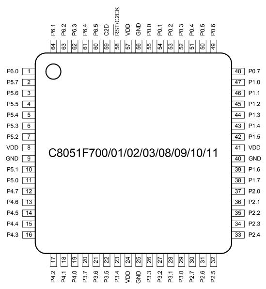
Figure 3.1. C8051F7xx-GM TQFP64 Pinout Diagram (Top View)
