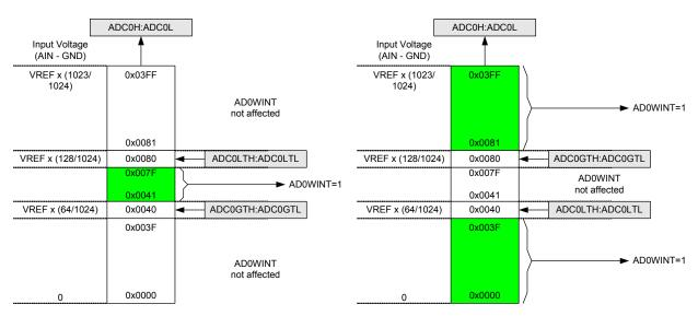
Figure 8.4. ADC Window Compare Example: Right-Justified Data
