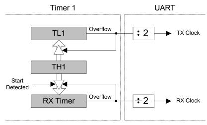
Figure 30.2. UART0 Baud Rate Logic
