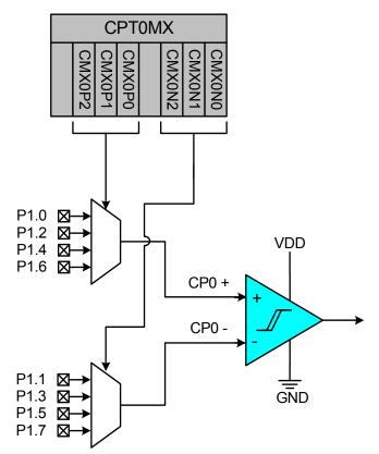
Figure 12.3. Comparator Input Multiplexer Block Diagram
