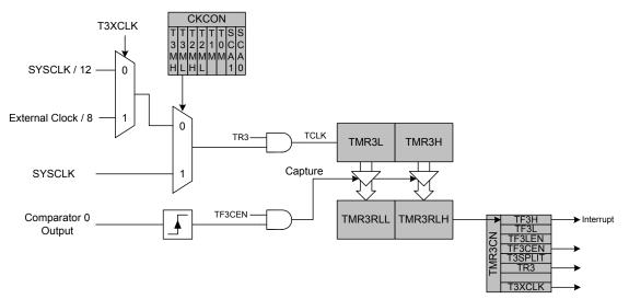
Figure 31.9. Timer 3 Capture Mode Block Diagram
