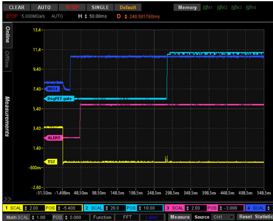
Figure 16-5. Startup Sequence Using [FASTADC] = 1 , with the [INITCOMP] Flag Displayed on the ALERT Pin.
