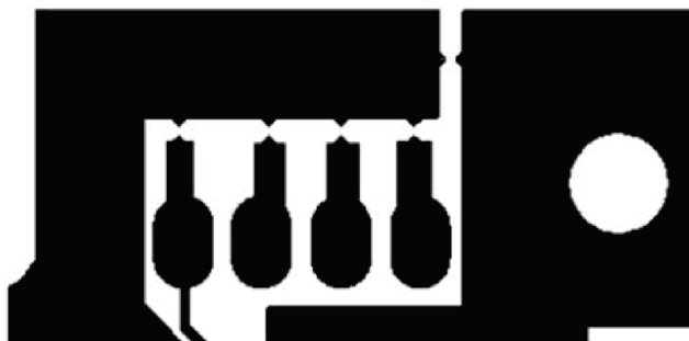
Figure 48. Recommended Spark-Gap Pattern Helps Protect Communication Lines from ESD
