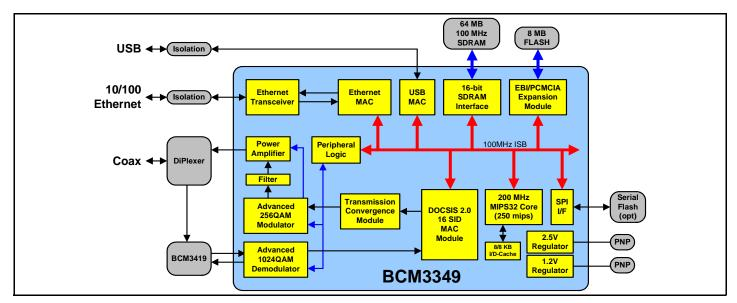
The BCM3349 combines an RF receiver with an advanced QAM and S-CDMA demodulator, an advanced QAM transmitter, a complete DOCSIS 2.0 Media Access Controller (MAC), a 200-MHz MIPS32 communication processor, a 16-bit, 100-MHz SDRAM interface, 10/100 Ethernet MAC with integrated transceiver and MII Interface, and a USB MAC with integrated transceiver.
