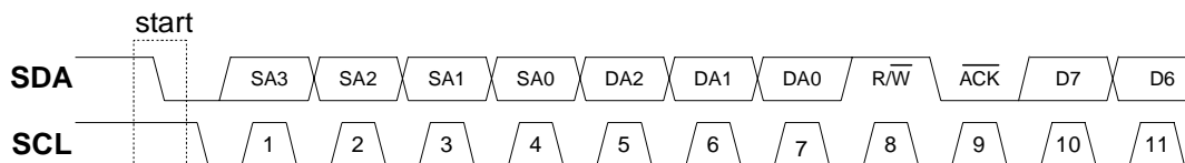
Figure 4-6. Addressing an I 2 C Peripheral
