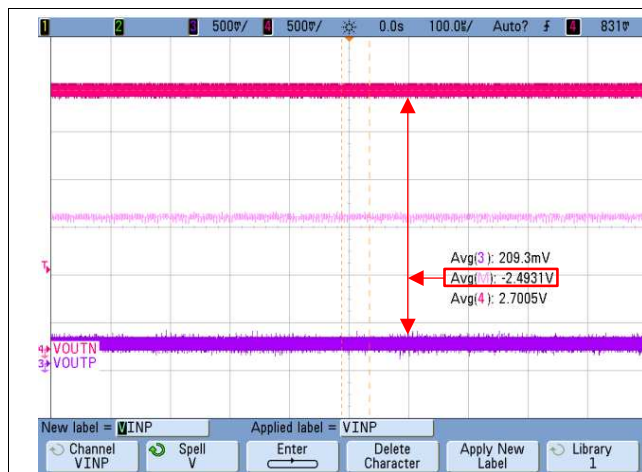
Figure 47. Typical Negative Clipping Output of the AMC1301-Q1 Device
