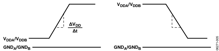
Figure 14. Transient Immunity Waveforms—Output Supplies
