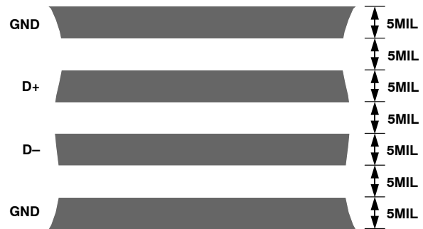
Figure 21. Typical Arrangement of Signal Tracks
