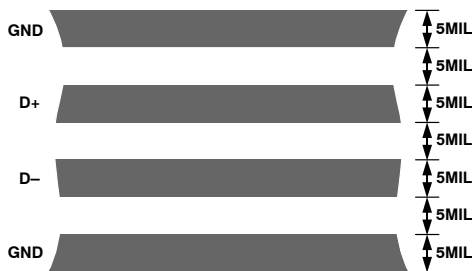
Figure 28. Arrangement of Signal Tracks
