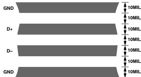
Figure 19. Arrangement of Signal Tracks
