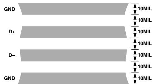
Figure 13. Arrangement of Signal Tracks
