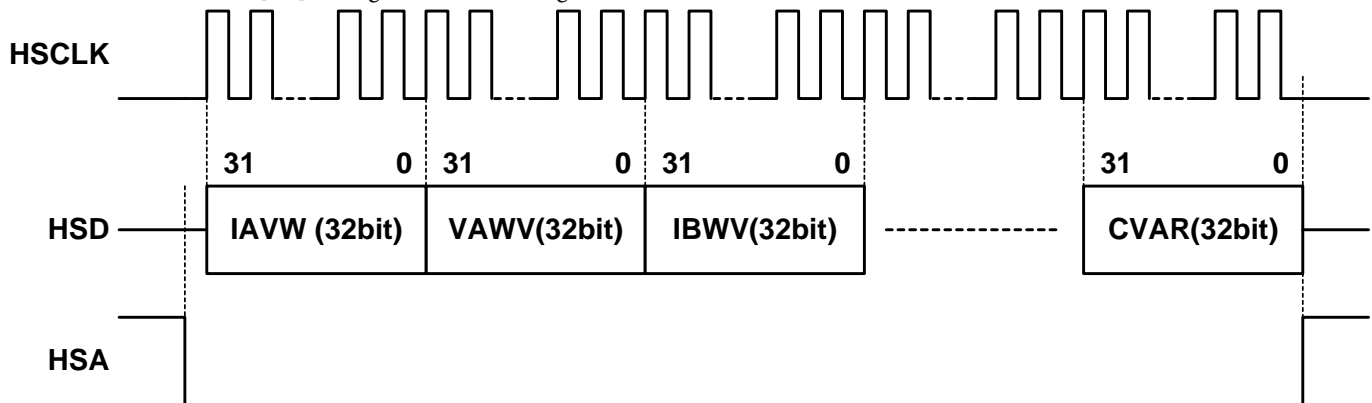
Figure 66. HSDC communication for HGAP=0, HXFER[1:0]=00 and HSAPOL=0. HSIZE is irrelevant
