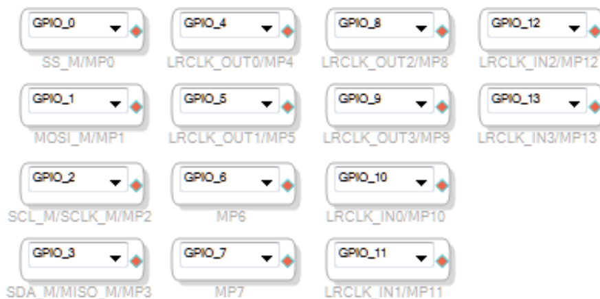
Figure 75. Complete Set of General-Purpose Inputs in SigmaStudio
