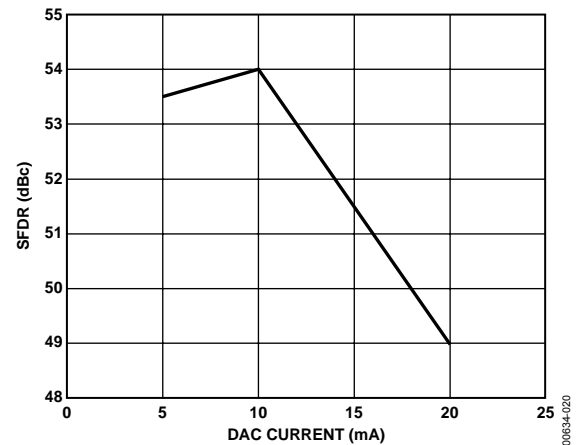
Figure 20. SFDR vs. DAC Current, 59.1 A OUT , 300 MHz REFCLK with REFCLK Multiplier Bypassed
