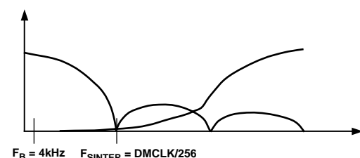
c. Digital Decimator Transfer Function
