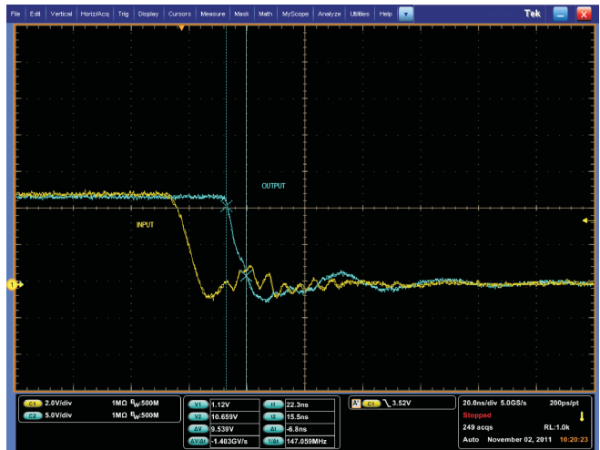
Figure 37. Turn-Off Fall Time ( C_L = 1.8 \text{ nF} , V_{DD} = 12 \text{ V} )
