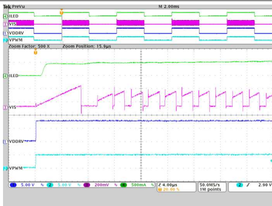
Ch1: DDRV voltage; Ch2: PWM input; Ch3: Switch sense current resistor voltage; Ch4: LED current; Time: 4 \mu s/div Figure 39. PWM Dimming Transient (Zoomed)
