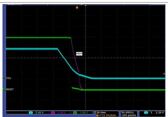
Figure 24. TPS7B6750-Q1 Power-Down Waveform
