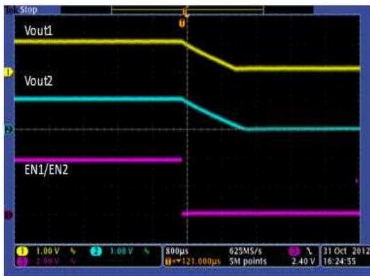
Figure 22. Shutdown With Enable
