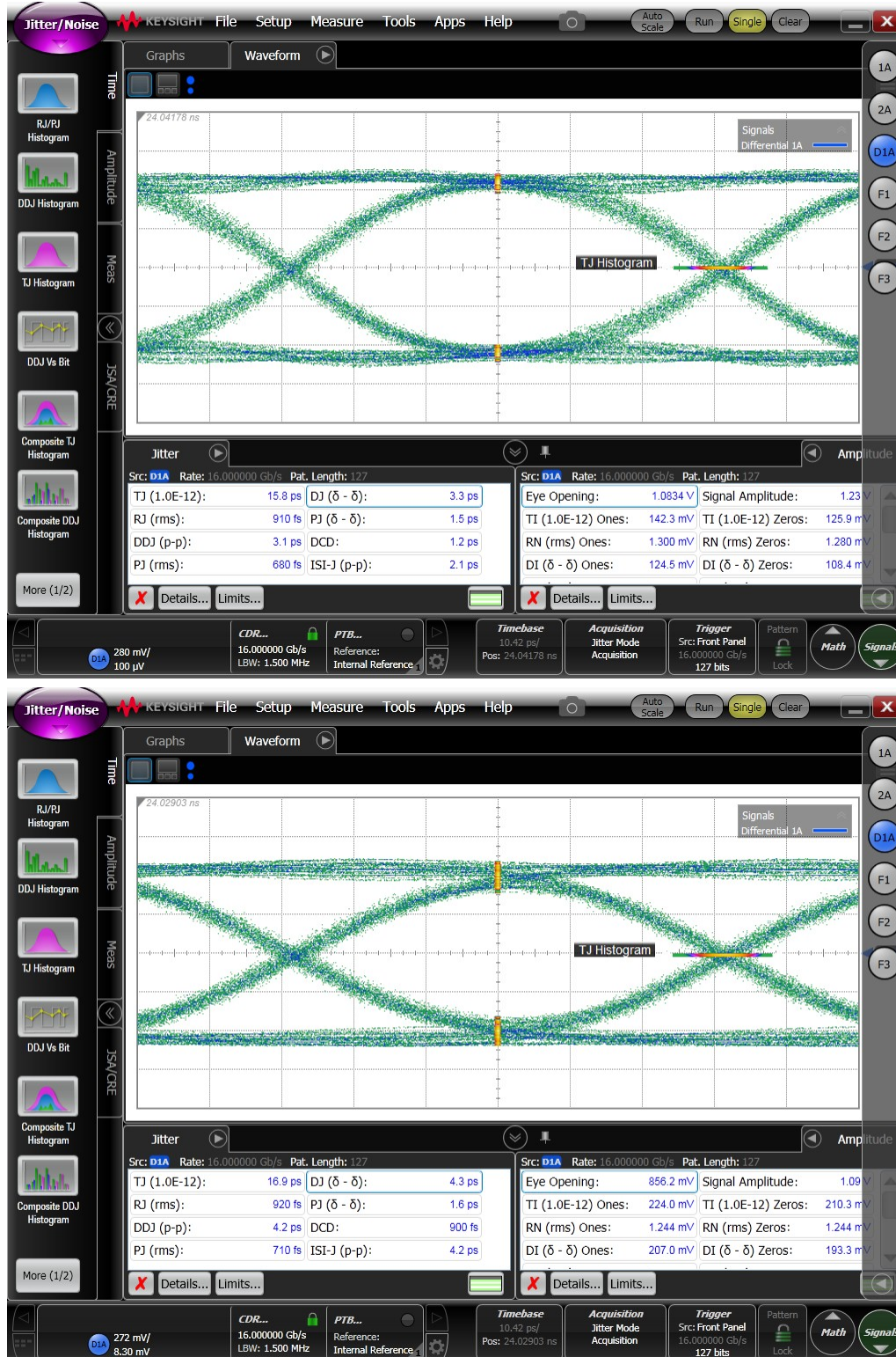
Figure 8-5. 16 Gbps PRBS-7 signals in TI evaluation board - Top: through calibration traces, Bottom: through a typical TMUXHS4412 channel
