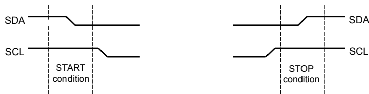
Figure 21-3. START and STOP Conditions
