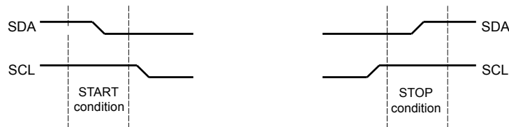
Figure 21-3. START and STOP Conditions
