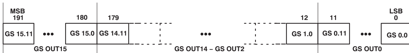
Figure 19. Grayscale Data Packet Format
