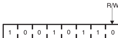
Figure 6. Software Reset Address
