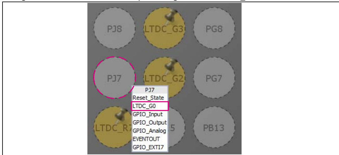
Figure 37. STM32CubeMX: PJ7 pin configuration to LTDC_G0 alternate function
