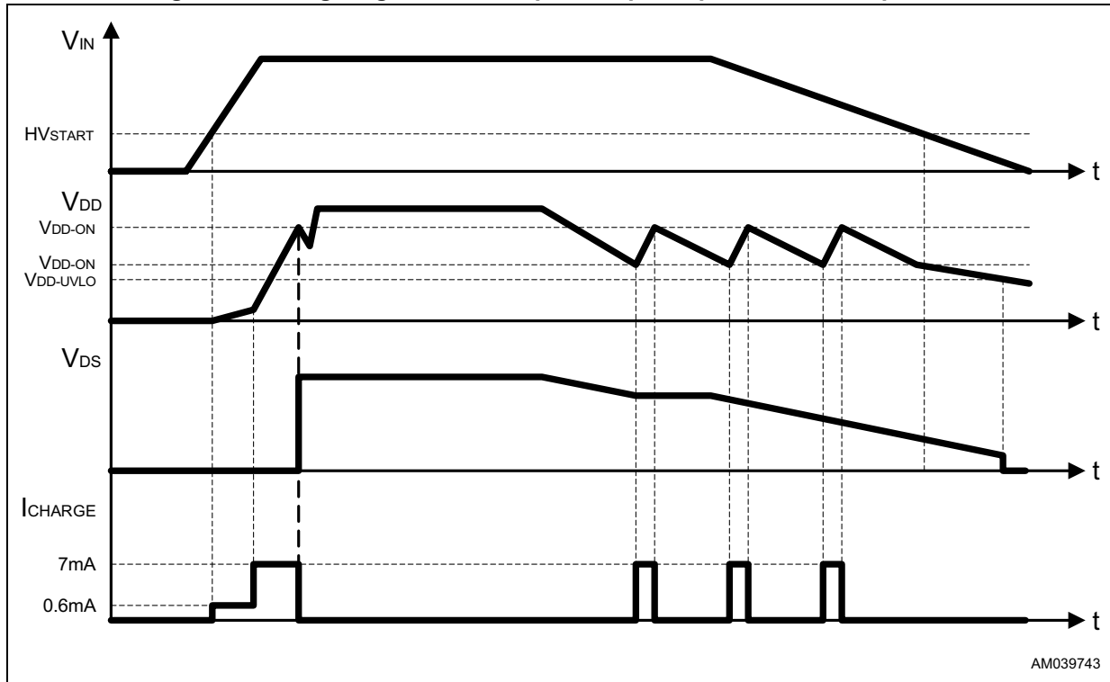
Figure 6. Timing diagram: normal power-up and power-down sequences
