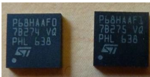
Figure 8: Picture of the Cryptographic Module (VQFN32) – Marking
