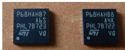
Figure 4: Picture of the Cryptographic Module (VQFN32) – Marking P68HAHB7 & P68HAHB8
