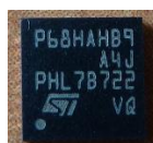
Figure 6: Picture of the Cryptographic Module (VQFN32) – Marking P68HAHB9
