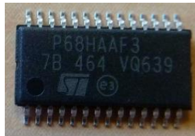
Figure 9: Picture of the Cryptographic Module (TSSOP28) – Marking
