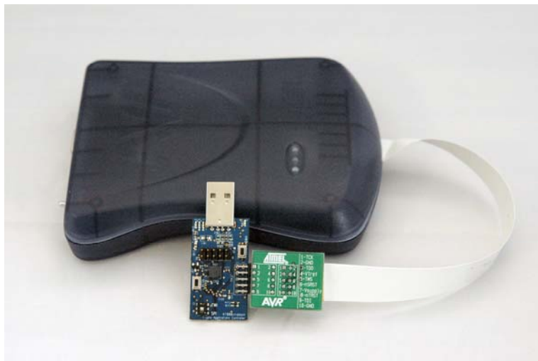
Figure 20. Connecting AVR JTAGICE mkII to the AT88Microbase
