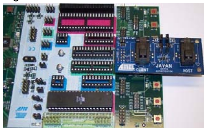
Figure 18. AT88CK109BK3 Mounted to the STK500
