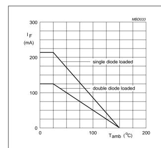
Device mounted on an FR4 printed-circuit board.
