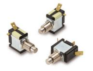
These rugged pushbutton-type switches feature international approvals, ratings to 20A 125VAC and a heavy actuation force (3-5 lbs. typical) which makes this switch ideal for use as a "foot-pedal" switch. These switches have become mainstays for canister Vacuum Cleaner applications. The metal bushing and plunger construction enables this alternate action switch to withstand the rigors of most any stringent pushbutton application.
