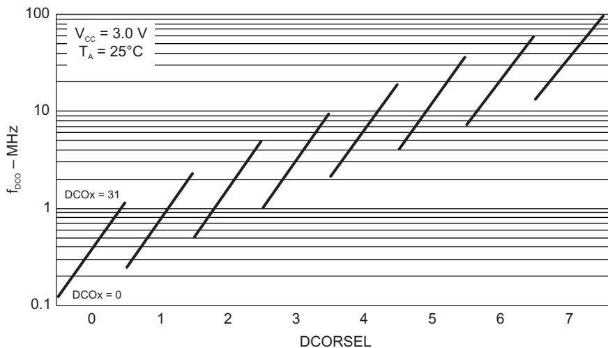
Figure 5-6. Typical DCO Frequency
